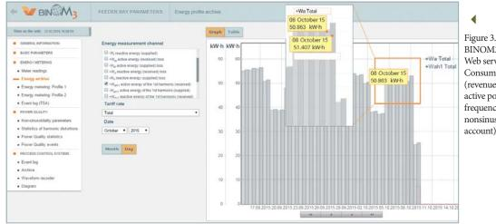
BINOM337U3.220I3.5S16T2 Web server: Daily Energy Consumption Histogram (revenue metering channels: active power at fundamental frequency, active power with nonsinusoidality taken into account)
