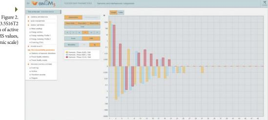
BINOM337U3.220I3.5S16T2 Web server: Histogram of active harmonic power (RMS values, odd order, logarithmic scale)
