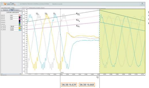
Figure 6. BINOM338U3.220I3.5 Web Server: Phase Voltage Waveform Combined with THD Chart (RMS values)
